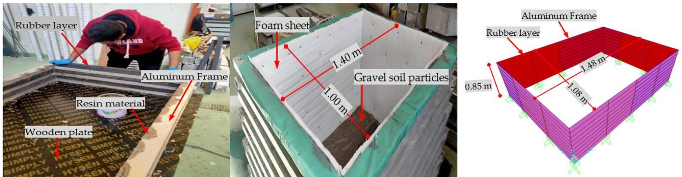
Figure 5. Constructed laminar shear box.
